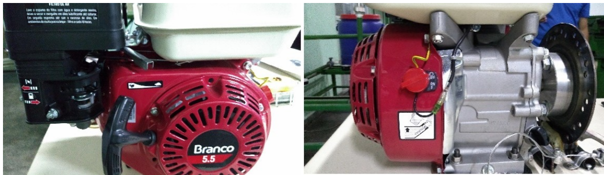
Figura 11: Motor Branco B4T – 5.5 HP.
