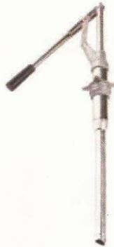
50305491 - BOMBA MANUAL P/TRANSFERENCIA LIQUIDOS; ACIONAMENTO: ALAVANCA; MATERIAL: ACO CARBONO; USO RESERVATORI: P/ TAMBOR 200L; TIPO FLUIDO: USO C/ OLEO DIESEL/LUBRIFICANTE; VAZAO: 250ML/CICLO; LUPUS: 90090S;
