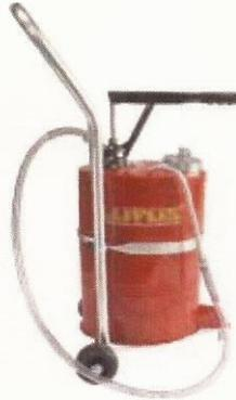
50305730 - BOMBA MANUAL P/TRANSFERENCIA LIQUIDOS; ACIONAMENTO: ALAVANCA; MATERIAL: ACO CARBONO; TIPO FLUIDO: USO C/ OLEO; VAZAO: 125ML/CICLO; LUPUS: 9005C; LUPUS EQUIP: 9005C;
